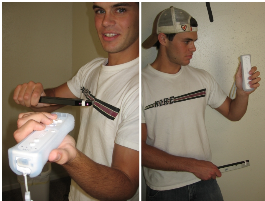
Figure 1: The orientation of the Wii remote determines whether the Wiiolin performs as a violin or cello
